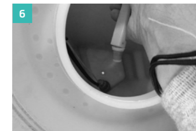
Open the plug on the water tank behind and leave open whenever the campervan is parked.
