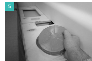
Open the blue cover on the water tank.
