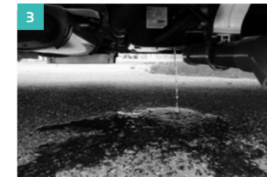
Check that water is coming out of the hot water tank under the left side of the van.
