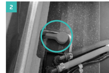
Turn the yellow knob under the rear seats to open and drain the hot water tank.
